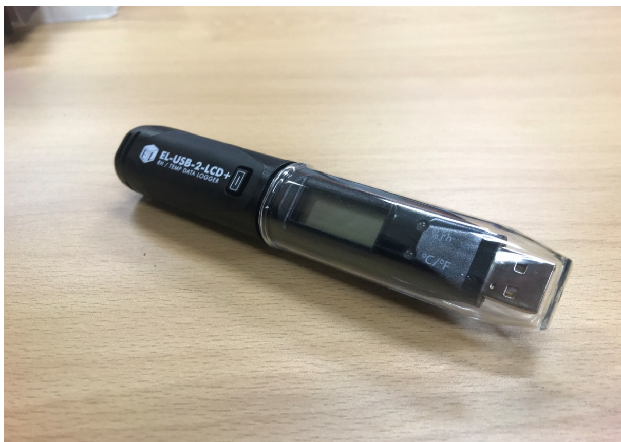
Figure S3. Portable sensor (EasyLog USB) for measuring the temperature ( ^{\circ}\text{C} ) and relative humidity (%).
